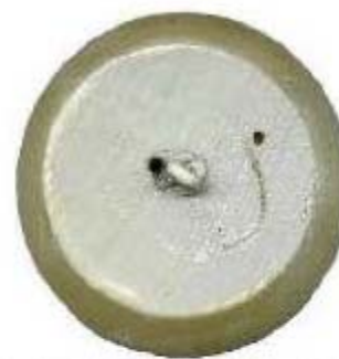
NOTE SAW/GRINDING MARKS, VERTICAL HOLE & BUBBLE
